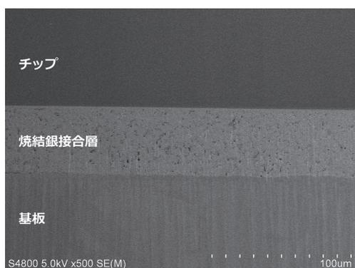
Figure 6 Cross-sectional SEM image of a sintered silver layer prepared with Bando FlowMetal® after 1000 cycles of a 200/−40°C thermal cycle test.
