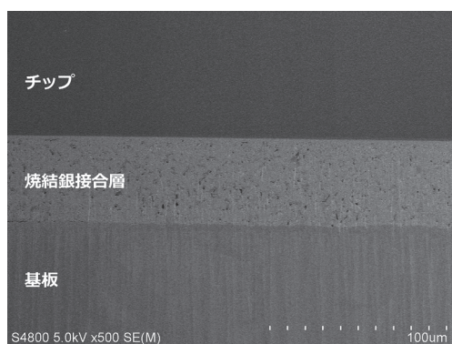
Figure 6 Cross-sectional SEM image of a sintered silver layer prepared with Bando FlowMetal® after 1000 cycles of a 200/−40°C thermal cycle test.
