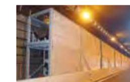
Pipe conveyor belt installed along expressway shoulder
