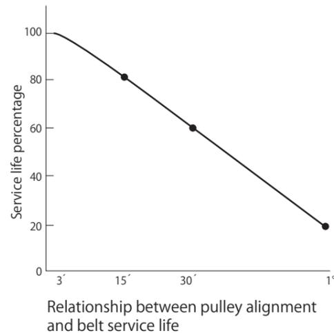
Hence, adjust the pulley alignment correctly based on **Table 8** before using a belt.
